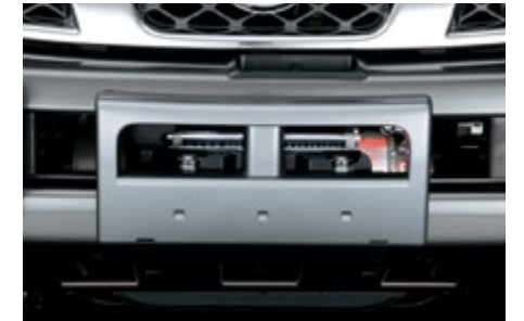
Winch An electric-powered winch, integrated with the front bumper, is very useful in emergencies.
