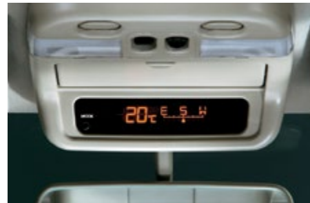
Multi-meter A digital multi-meter, positioned between the sun visors, displays the outside temperature and compass direction.
